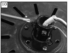
Loosen the 2 set screws in yoke for downrod to slip into yoke.
